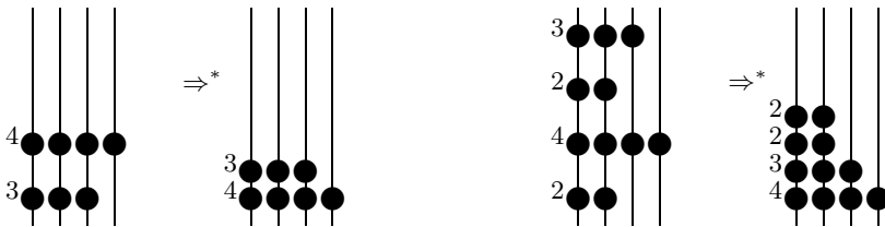
Fig. 4. Sorting the sets \{4, 3\} and \{3, 2, 4, 2\} using beads that slide on rods.
